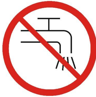
Figure 104 – Warning symbol: Machine not suitable for connection to the potable water mains
